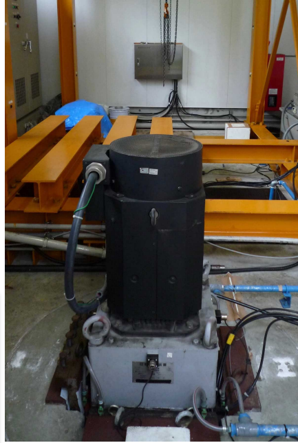
Continuous observation of seismic wave velocity and apparent velocity using a precise seismic array and ACROSS seismic source
