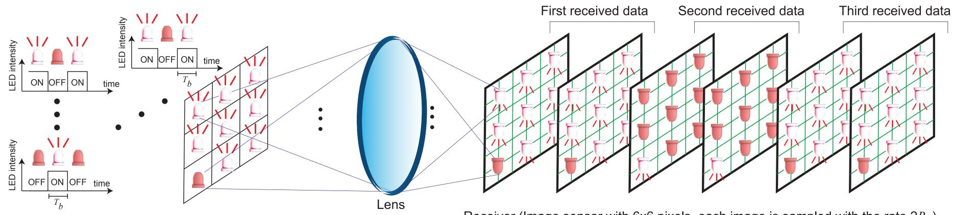
Transmitter (3x3 LEDs alligned in a grid (LED array))
