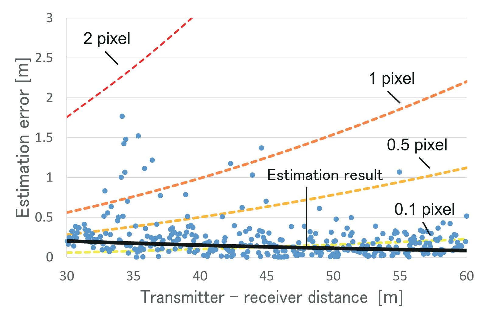
The range estimation error plots along with numerically obtained error curves assuming sub-pixel error. The curves labeled 2-pixel and 1-pixel are the case without POC while the curves labeled 0.5-pixel and 0.1-pixels are the case with POC. The black solid curve is the approximate curve of the range estimation (plots).
