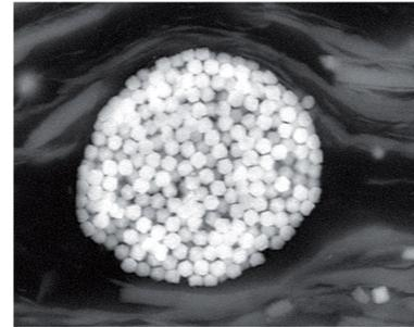
Indirect precipitation of pyrite ( $FeS_2$ ) by sulfate-reducing bacteria
