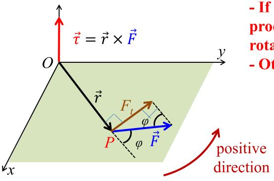
If the torque tends to produce a counterclockwise rotation, it is PositiveOtherwise, it is negative.
