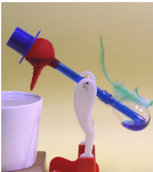
11-5 (a) Drinking Bird as a Heat Engine
